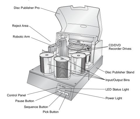
The **Robotic Arm** transports discs from an Input Bin, to a CD/DVD Recorder, to the printer, and finally to an Output Bin.
